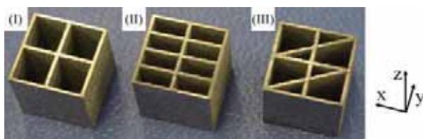
Fig. 10 SLMed specimens produced from quadrangular prismatic structural CAD models as shown in Fig. 9(I), (II) and (III).
