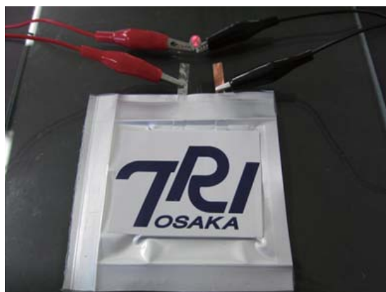
Fig. 8 An image of the laminated all solid state battery prototype under development.
