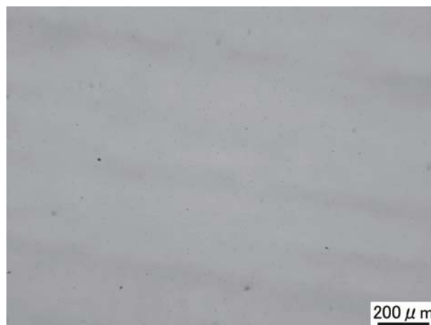
Fig. 9 Optical micrograph of a horizontal cross section of an SLM specimen fabricated under the optimum laser irradiation conditions.
