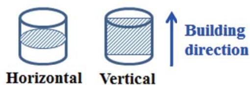
Fig. 3 Horizontal and vertical cross sections for microstructural observation.
