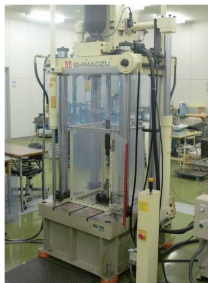
Fig. 4 High-speed impact testing machine.
