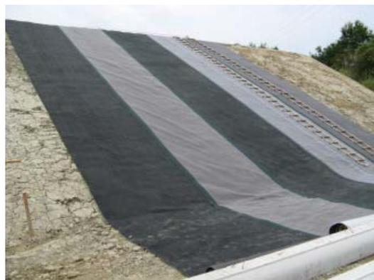
Fig. 4 GCs laid on the test slope.
