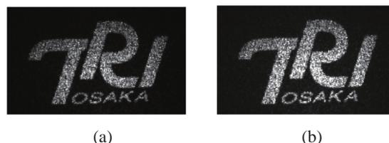
Fig. 7 Reconstructed images of master pattern (a) and replica pattern (b). These images were captured by CCD camera when master pattern and replica pattern were illuminated with a He-Ne laser, respectively.
