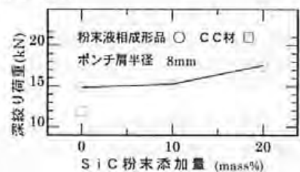
図9 深絞り荷重に及ぼすSiC粉末添加量の関係 (O材) Effect of the amounts of SiC-particles on deep drawing pressure
