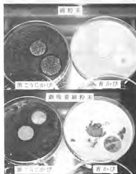
図 4 綿粉末および銀吸着綿粉末のかび抵抗性 Fungus resistance of cotton powder and silver adsorbed cotton powder
